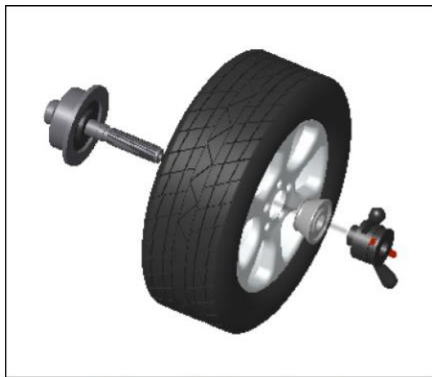
Main shaft--wheel (Installing face of rim forward inside) Cone (tip pointing to inside)--fast clamp
